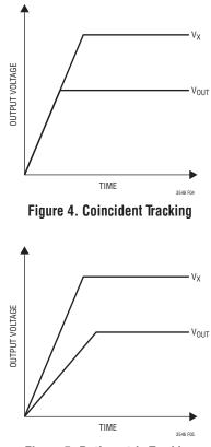
Figure 5. Ratiometric Tracking
