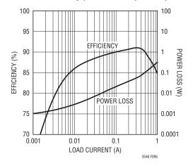
OUT2 Efficiency (Burst Mode Operation)
