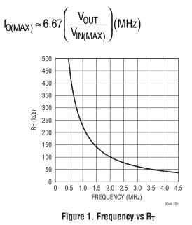
The minimum frequency is limited by leakage and noise coupling due to the large resistance of  $R_{T}$ .
