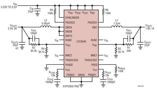
Figure 9. Typical Schematic for 3A/1A Regulator
