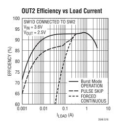
OUT2 Efficiency vs Load Current
