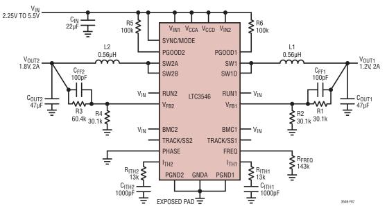
Figure 7. Typical Schematic for 2A/2A Regulator
