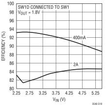
OUT1 Efficiency vs V<sub>IN</sub>
